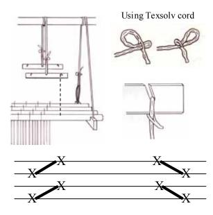
Counterbalance tie-ups require that the cords are positioned to make a symmetrical tie-up, as in the diagram.
