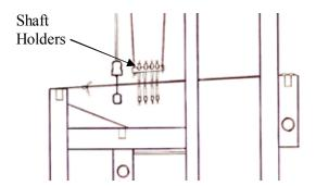
The warp travels in a straight line from the back beam to the breast beam. See page 6 for setting the shafts and beater at the correct height.
