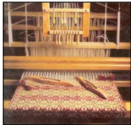
Opphamta attachment with 10 pattern shafts, 1970s
