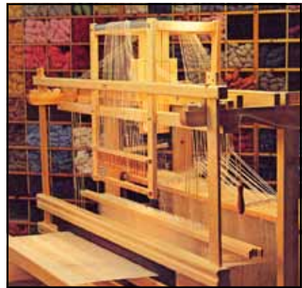
Opphamta attachment With 20 pattern shafts, can be used with a countermarch tie-up
