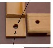
This is because the 'cap' fits in the larger hole and the screw part in the smaller. Insert the cap and then the screw and assemble using the hex key. Do each corner but *remember* to insert the MIDDLE bar into the mortises with the hooks pointing to the edge of the frame
