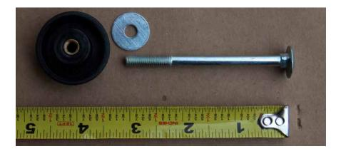
The long bolt is about 3 inches long and is used to attach the back legs of the stand to the loom and heddle bracket. The washer is on the outside. Use the black knob to secure the assembly.
