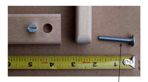
On the cross piece there generally is no washer. The short (about 1.75 inches) flat headed bolt is used. Line up the slot in the barrel with the bolt when assembling.
