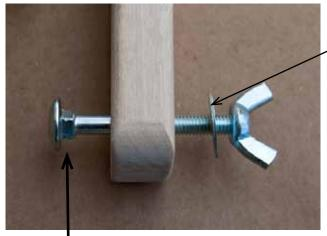
Washers typically are placed between the nut (wing nut or knob) and the wood. The threaded portion of the bolt typically points to the outside of the loom or stand or frame
