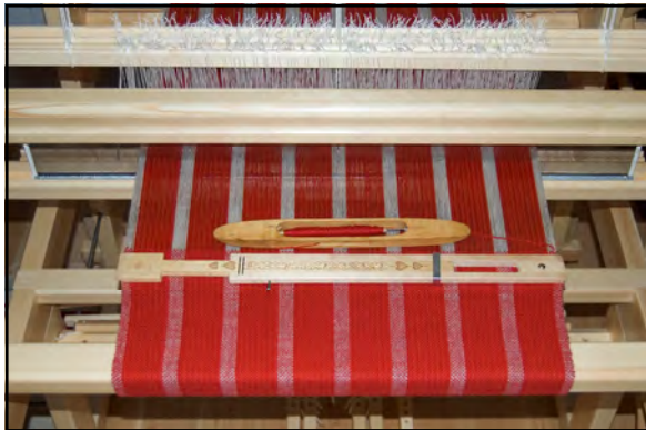
Red blanket being woven with a long damask shuttle with a 6 inch quill, on a 39 inch loom
