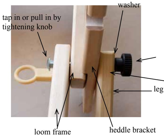
the longer leg of the 'X' frame attaches at the bracket. Remove the shorter bolts and replace with longer bolts, supplied.
