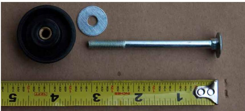
The long bolt is about 3 inches long and is used to attach the back legs of the stand to the loom and heddle bracket. The washer is on the outside. Use the black knob to secure the assembly.
