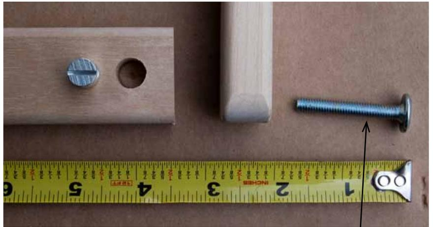
On the cross piece there generally is no washer. The short (about 1.75 inches) flat headed bolt is used. Line up the slot in the barrel with the bolt when assembling.
