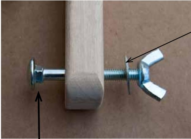
Washers typically are placed between the nut (wing nut or knob) and the wood. The threaded portion of the bolt typically points to the outside of the loom or stand or frame
