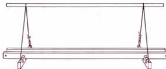
Shaft holders assembled with Texsol cord.
